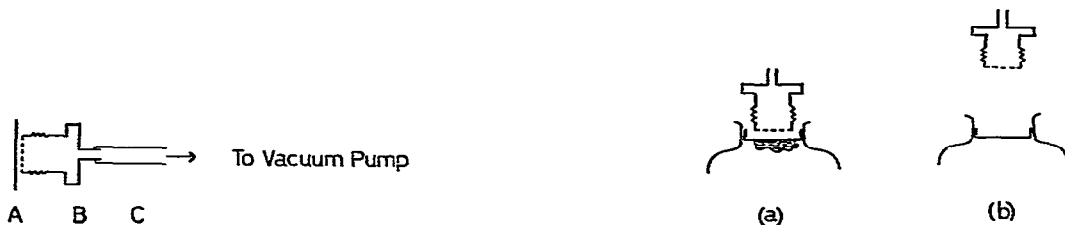
Fig. 1. Vacuum recovery device. A = Whatman No. 1, 2.1-cm filter paper disc; B = the "male" half of a 1.3-cm diameter Sartorius Syringe Filter Holder (V. A. Howe, London, Great Britain); C = flexible plastic tubing.
